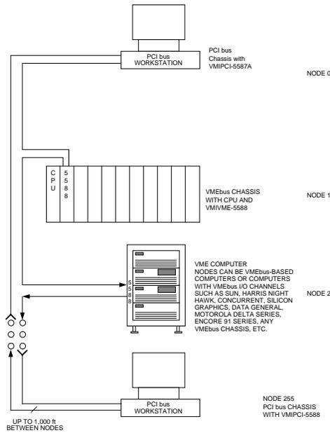
**Figure 1. Network Example Using Reflective Memory System**
