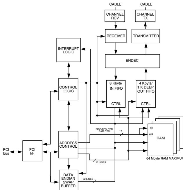
**Figure 2. VMIPCI-5587A Functional Block Diagram**
